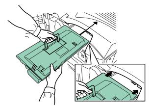
When inserting, be sure that the gear side of the toner container faces the printer. Leave the front cover open to allow insertion of the waste toner box.
